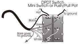
Optional: Series / Parallel Wiring yields a more "open" tonal effect. Use a DPDT push/pull pot or mini toggle switch.)
